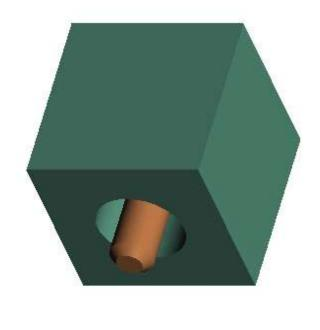
Imperfections in geometry and clearances between parts cause undesirable adjustments within assemblies
